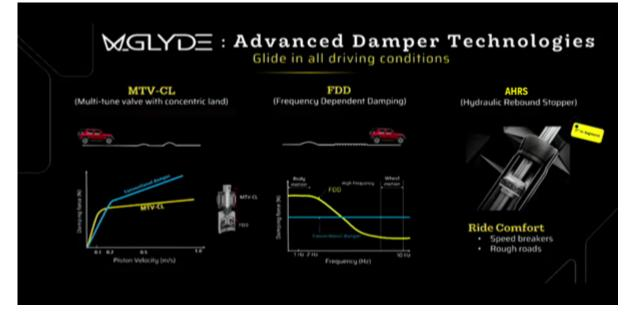
The 2024 Mahindra Thar ROXX from Mahindra and Mahindra Ltd. is the first new passenger vehicle to feature Monroe OE Solutions passive dampers fitted with Tenneco's Monroe Ride Refine<sup>™</sup> <u>Advanced Hydraulic Rebound Stop</u> (AHRS), which minimizes suspension rebound topping energy and noise during offroad driving and in other extreme environments.
